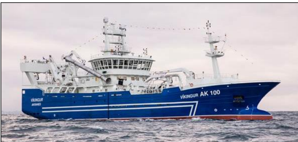
Figure 11. An example of a large combination purse-seiner/pelagic trawler in the Icelandic fleet operated by HB Grandi (Vikingur AK 100; built 2015; 81 m LOA; 3,672 GRT) (Source: http://www.hbgrandi.com/ ).
